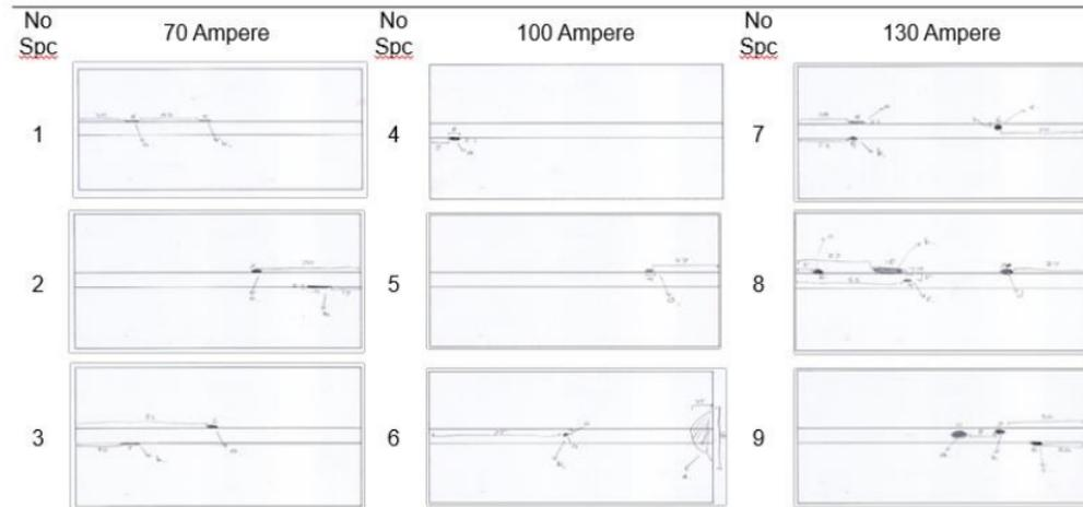
**Gambar 1.3** Hasil Analisa Liquid Penetrant Testing
