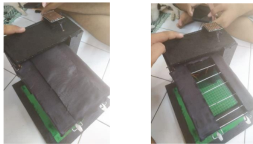
Fig. 11. Condition Cloudy but roof can still be opened by telegram
