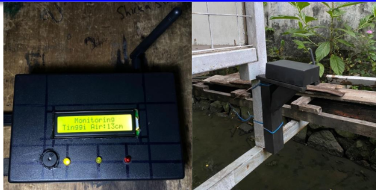
Fig 8. Displays a safe condition because the water level is < 25 cm
