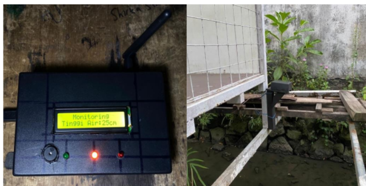
Fig 9. Displays an alert condition because the water level is 25cm
