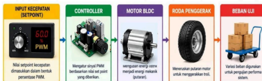
Gambar 2.3 Diagram Blok Sistem Kontrol Open-Loop Motor DC
