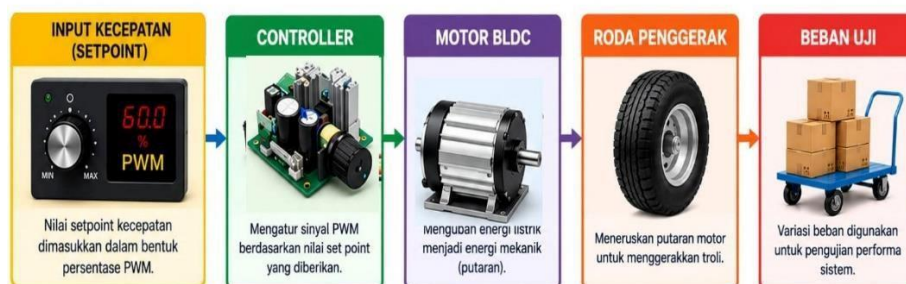
Gambar 2.3 Diagram Blok Sistem Kontrol Open-Loop Motor DC
