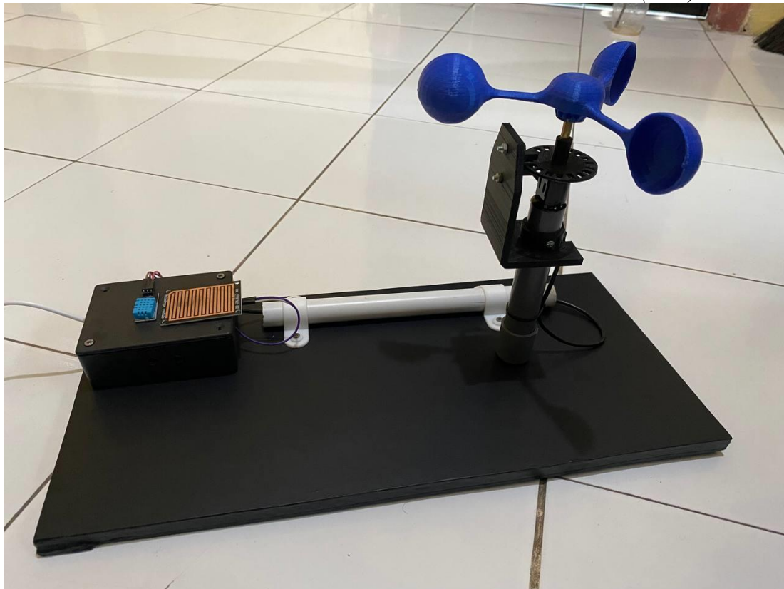
GAMBAR 3.2 HARDWARE MONITORING CUACA
