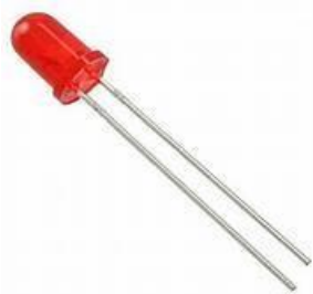
Gambar 4. LED Indicator Sistem Early Warning
