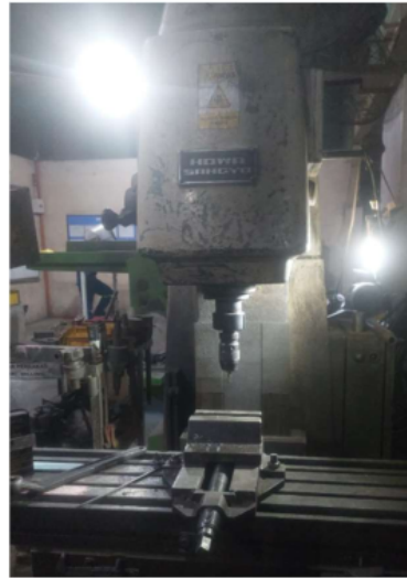
Gambar 2 Mesin Frais Universal HOWA SANGYOU
