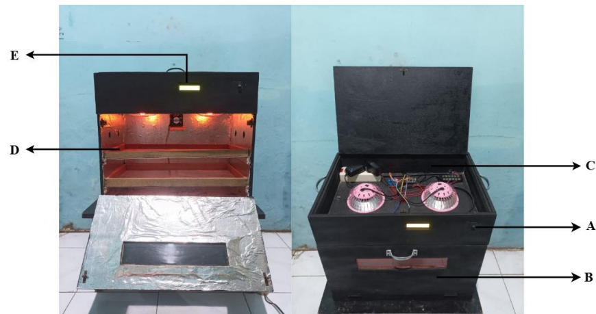
Gambar 4. Prototype Inkubator Monitoring Suhu dan Kelembaban
