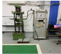
Gambar 8. Alat Uji Tarik Universal Testing Machine (UTM) merek Tarno Grocki
