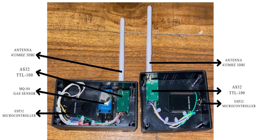
Gambar 2. Implementasi fisik unit transmitter dan receiver
