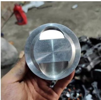
Gambar 1. Piston berdiameter 68 mm
