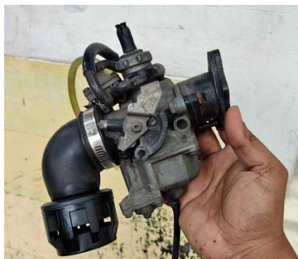
Gambar 8. Karburator OEM honda megapro
