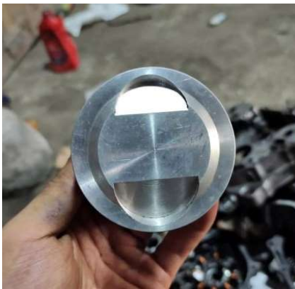
Gambar 1. Piston berdiameter 68 mm
