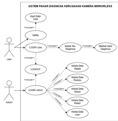
Gambar 2. Use Case Diagram
