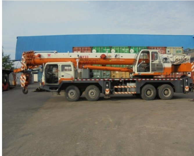
Gambar 1. Mobil Crane Zoomlion 55 ton
