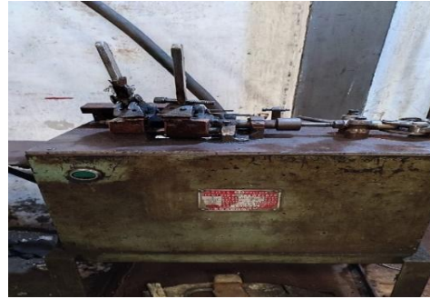
Mesin Flash Butt Welding (FBW)
