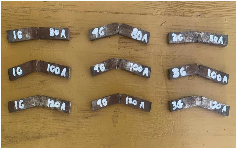
Hasil Pengujian Impak Pengelasan 1G, 3G dan 4G SMAW (Shielded Metal Arc Welding)
