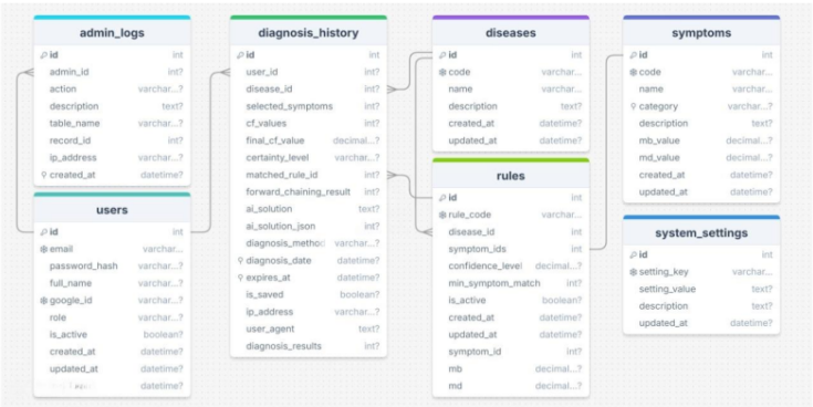
Gambar 4. Entity Relationship Diagram (ERD)
